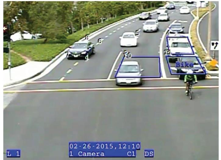
Bicycle zones are placed in bike lanes (left) as well as in vehicle lanes, including the left turn lane (right). Bicycles are detected and uniquely identified as “Bike” while regular motor vehicles are detected normally.
